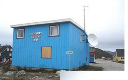
were pointed nearly parallel with the surface of the earth to make contact with satellites over the equator.
